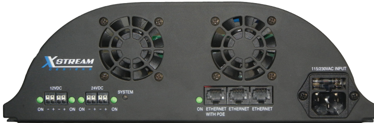
Figure 1.1 - X|Smart_PSP Power Supply Chassis
