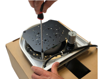
Figure 14 - Securing camera mount assembly to the standoffs.
