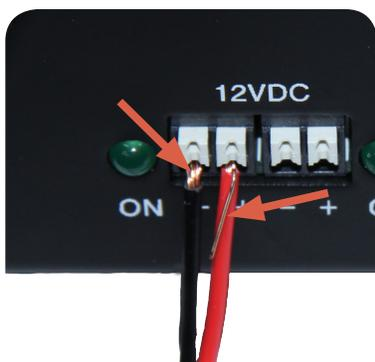
Figure 5.6 - Exposed Wire & Poor Connection
