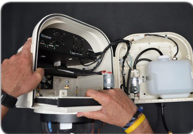
Figure 8.3 - Removing the camera tray.
