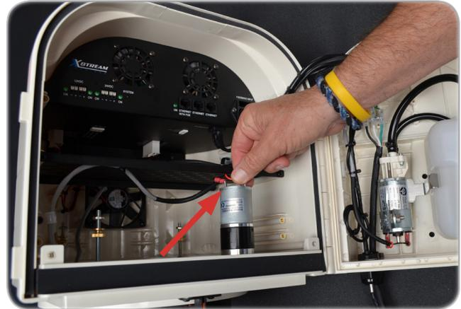
Figure 8.2 - Disconnecting the motor cables.
