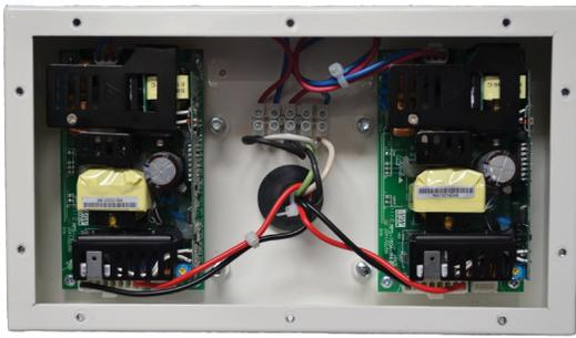
Figure 5.1 - X|Cold External 15VDC Power Supplies
