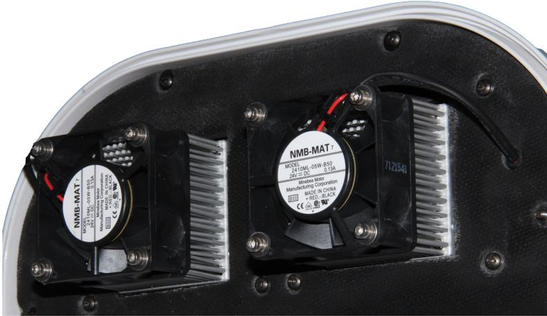
Figure 12.1 - X|Cold Solid State Cooling Components
