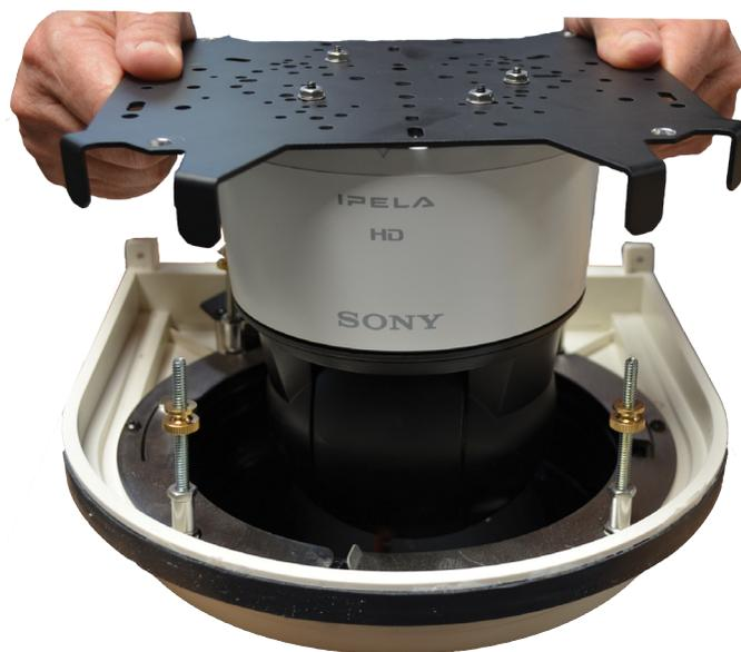
Figure 7 - Solid Camera Mounting
